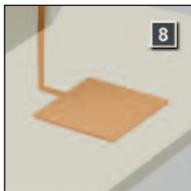
Choose an earth electrode to suit the system design i.e. Type A, Type B or foundation electrode. Electrodes can be constructed individually from earth rods, earth plates, flat tape, stranded cable or any combination of these.
