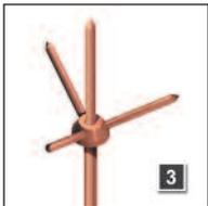
Use air terminals in the form of vertical air rods for the protection of prominent roof top features or equipment. Use strike pads to connect and thus expose concealed conductors.
