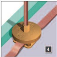
Choose the correct air rod base. This will ensure that the vertical air rods are both solidly fixed to the fabric of the structure and have a low resistance connection to the conductor network.
