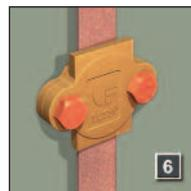
In order to allow periodic disconnection and testing of the earth termination network, select a test clamp to be placed within the run of each down conductor.
