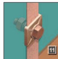
Select the correct type of metalwork bond for the application, i.e. a flat column face, a circular rainwater pipe or a ribbed reinforcing bar.
