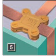
Select a component for the interconnection of multiple conductors or for changes of direction. Jointing clamps will ensure a low resistance, corrosion resistant connection between air termination and down conductors.
