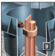
Select a high copper content alloy earth rod clamp for the connection of the earthing conductor to the earth rod. In this below ground application, the clamp must ensure a good electrical contact and resist corrosion throughout the lifetime of the installation.
